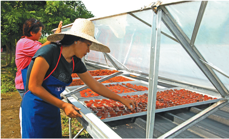
Members of a women's group in Nueva Ecija use the Multi-commodity Solar Tunnel Dryer to add value to their produce such as tomato.
